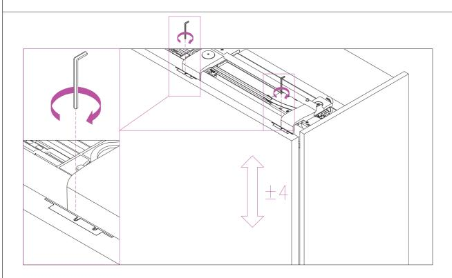
19 - Adjust the door vertically using a 3mm allen key working on the both the RD and R boxes.
