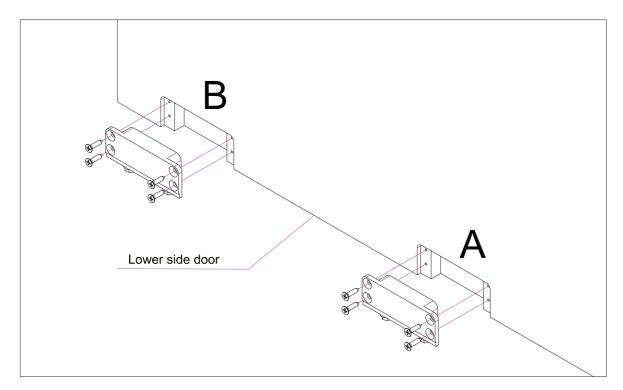
9 - Screw the block slider, put them in the seats in the lower side of the door
