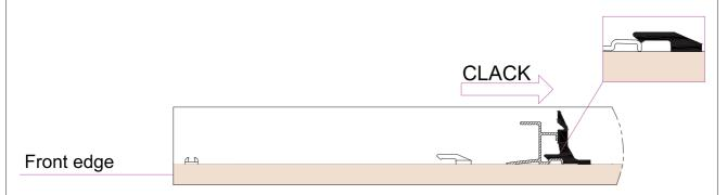
3 - Insert and ensure that the profile B couples with the clip
