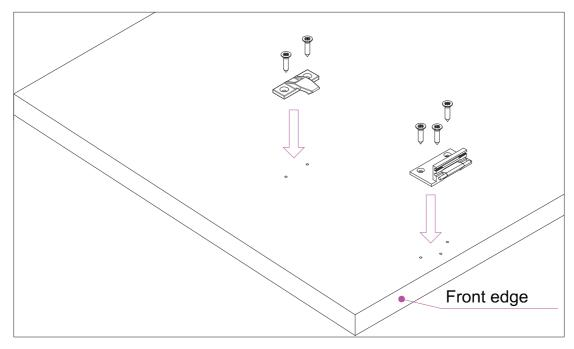
2 - Fix with self threading screws by the drillings
