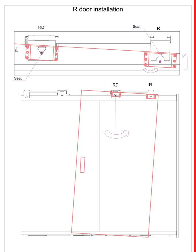
15 - Rotate the door until it couples with the pin by the R seat15a - Before starting with the assembly of the other doors, mount the sliders
