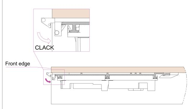
7 - Join the profile C to the sole panel in order to release the clip that definitely blocks the profile C
