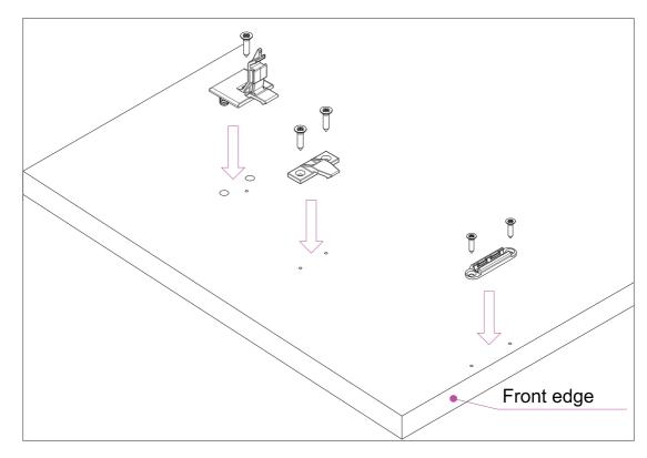
1 - Fix with self-threading screws by the drillings
