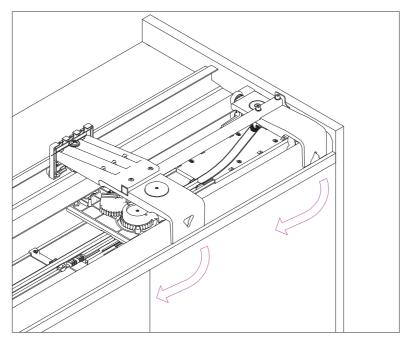
12 - Open the upper mechanism so that the coupling clamps open
