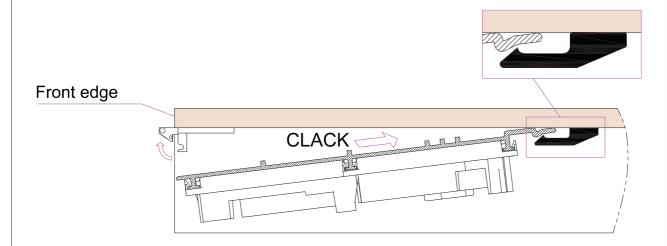
6- Ensure that the back lower clip is open6a - Insert the profile C slightly inclined and couple it with the back clip
