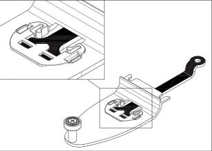
10 - Insert the key in the slider and hook it to the clip
