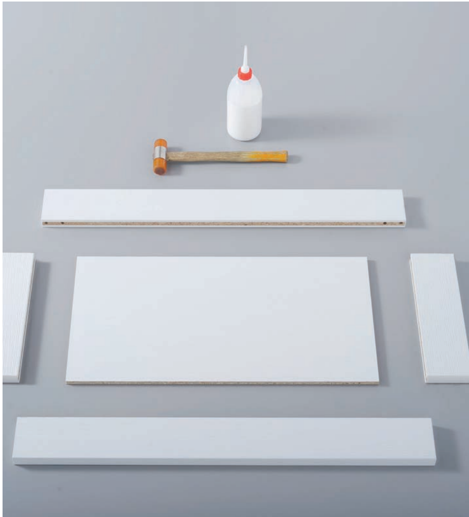
colla glue martello da falegname carpentry hammer montanti e traversi lateral posts and side beams pannello board spine plugs
